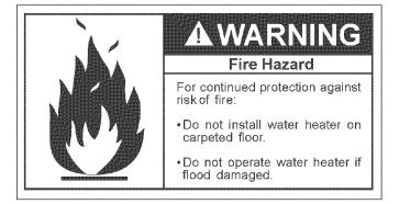
This water heater must not be installed directly on carpeting. Carpeting must be protected by metal or wood panel beneath the appliance extending beyond the full width and depth of the appliance by at least 3 inches (76.2 mm) in any direction, or if the appliance is installed in an alcove or closet, the entire floor must be covered by the panel. Failure to heed this warning may result in a fire hazard.
